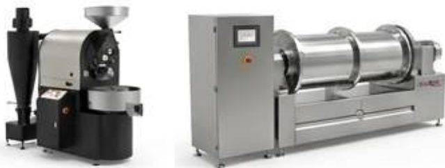
PACKINT integrated ball mill refining and conching systems for micro-particle reduction
